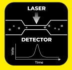
Counts and measures particles in predetermined particle size cuts
