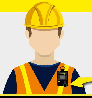
The dust sample is drawn into the DustCanary **TREND 420** through the inlet at the front of the device, ensuring accurate measurements representative of the air the wearer is breathing.
